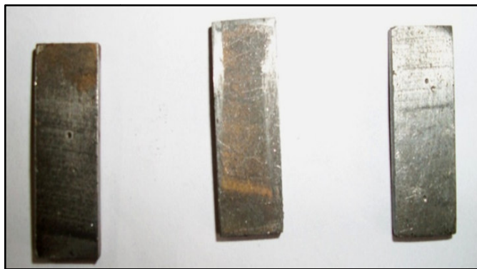
Fig.3: Hot pressed diamond cutting tools made by application of electrolytic iron powder
